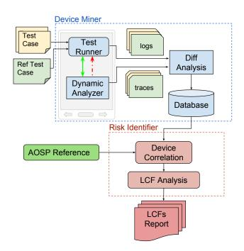
Fig. 1. Design of ADDICTED. Test cases are first executed by Test Runner and analyzed by the Dynamic Analyzer. The logs and traces are analyzed by the Diff Analysis tool to filter out irrelevant device operations and later sent to Risk Identifier to check for LCFs.
