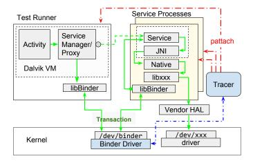
Fig. 2. Dynamic Analyzer. In the figure, the dashed green (---) line describes a conceptual RPC call and the solid green line (—) is the real call chain for accessing hardware devices. The dash-dash-dot red ( $-\cdot-\cdot-$ ) lines show how the tracer is attached to all the processes related to a device operation and the dash-dot blue (----) line illustrates how this attachment operation is performed by the binder.
